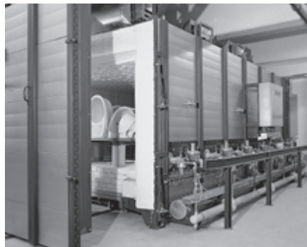
Intermittent shuttle kiln in the ceramics industry
